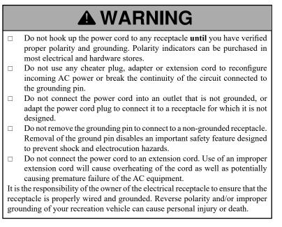
The 30-amp external utility power cord is commonly referred to as the "shore" power cord. It is designed to mate and properly function with 30-amp "shore" power receptacles available at most campgrounds.
