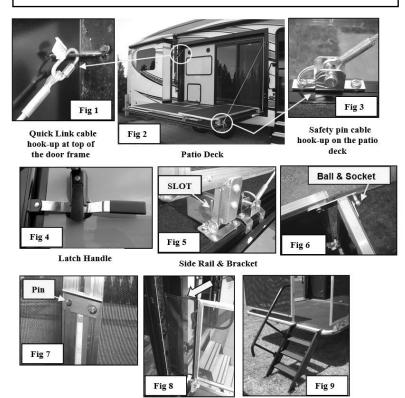
To set up the patio deck, unlatch the two keyed handles from the side of the RV (**Fig 4**). Lower the patio deck until the cables on each side support it. Support cables are attached at the top of the door opening with a quick link (**Fig 1**) and to the deck with a safety pin (**Fig 3**).
