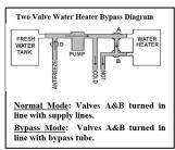
**<u>NOTE</u>**: In the diagram: Valve A is the black valve, valve B is the white valve. Valve D is the suction (siphon) valve that has the clear hose attached to it for siphoning in antifreeze, sanitizer or fresh water from an external container. This valve is typically located at the water pump.
