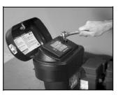
Use an electric drill with a 5/16" socket to manually raise or lower each rear leg.
